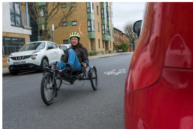
Recumbent cyclists have a lower seating position and reduced visibility envelope. Credit: photojB/Sustrans
